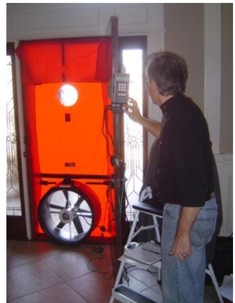
Figure 5 - Blower Door Apparatus
